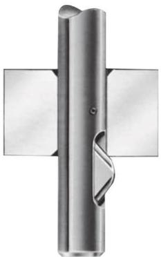
3. Spring tension again causes the blade to extend as it emerges from the ID of the part; the burr is removed on the back side of the hole on the return stroke.
