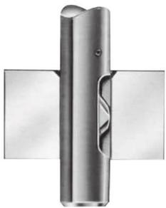
2. As the feed load increases, the pre-set spring tension is exceeded and the blade retracts automatically as the tool passes through the workpiece. (The crowned and polished top surface of the blade will not mar the inside surface of the hole.)
