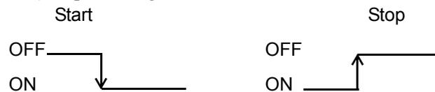
**6-5. External Output Signal****(1) Near Zero [ pin 17 ]**
