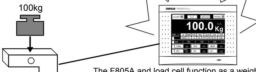
The F805A and load cell function as a weighing device.
