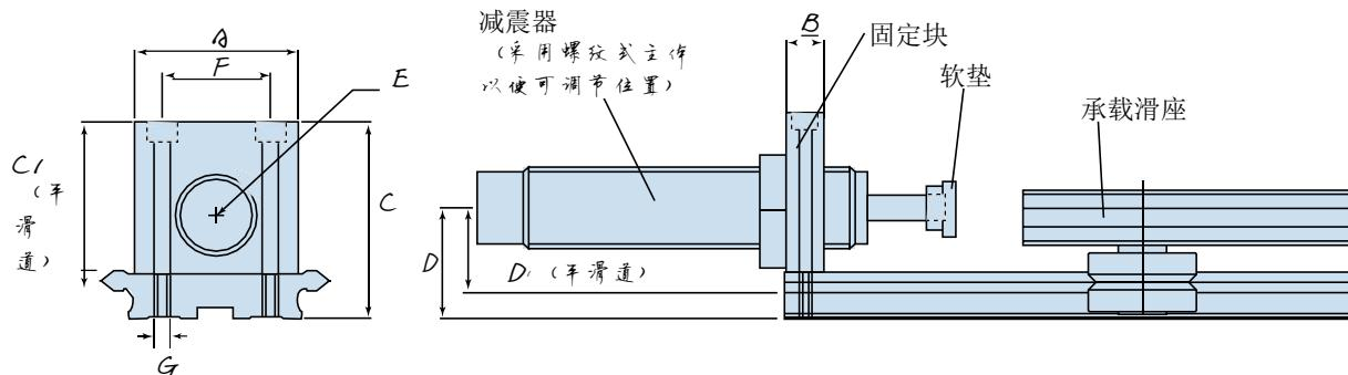
订购示例：NL120L1616P2 + 1 x SHBL12036 (1x = 一端固室内支架, 2x = 两端固室内支架)
