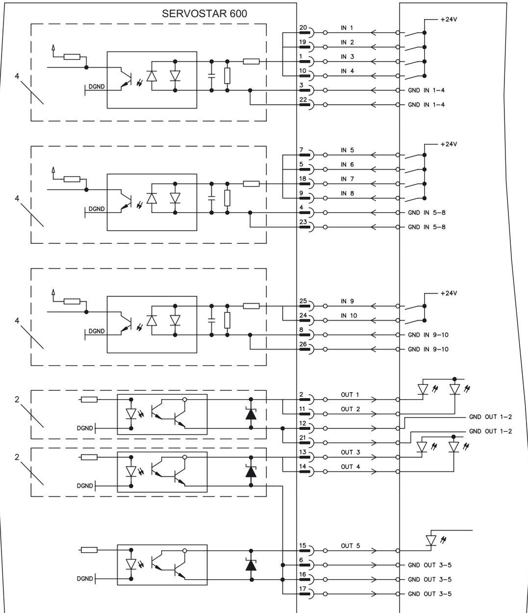
Pin assignments for connector X18 (SubD 26-pin)
