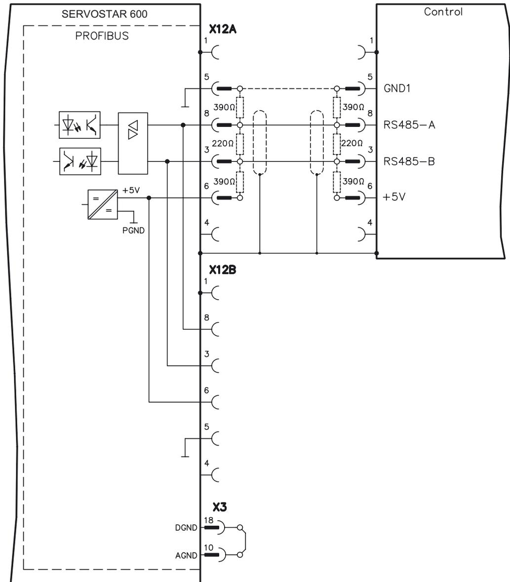
**AGND and DGND (connector X3) must be joined together !**
