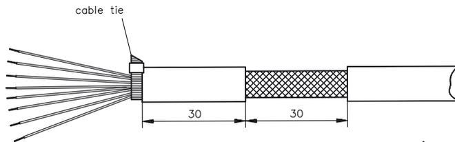
Remove the outer covering of the cable and the shielding braid from the cores for the required length. Secure the cores with a cable tie.
