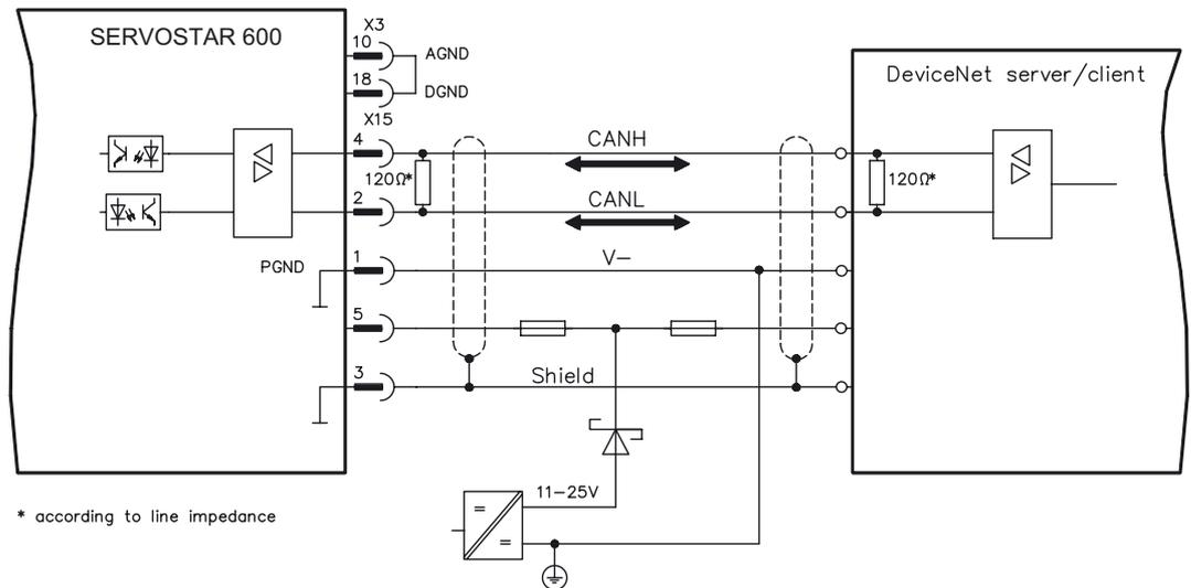
**AGND and DGND (connector X3) must be joined together!**
