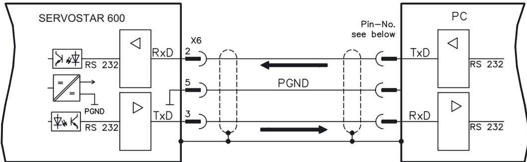
Interface cable between the PC and servo amplifiers of the SERVOSTAR 600 series:
