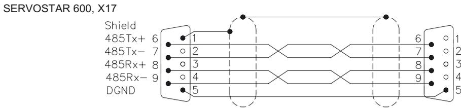
RS485 Half Duplex Modus is adjustable through the setup software DRIVE.EXE
