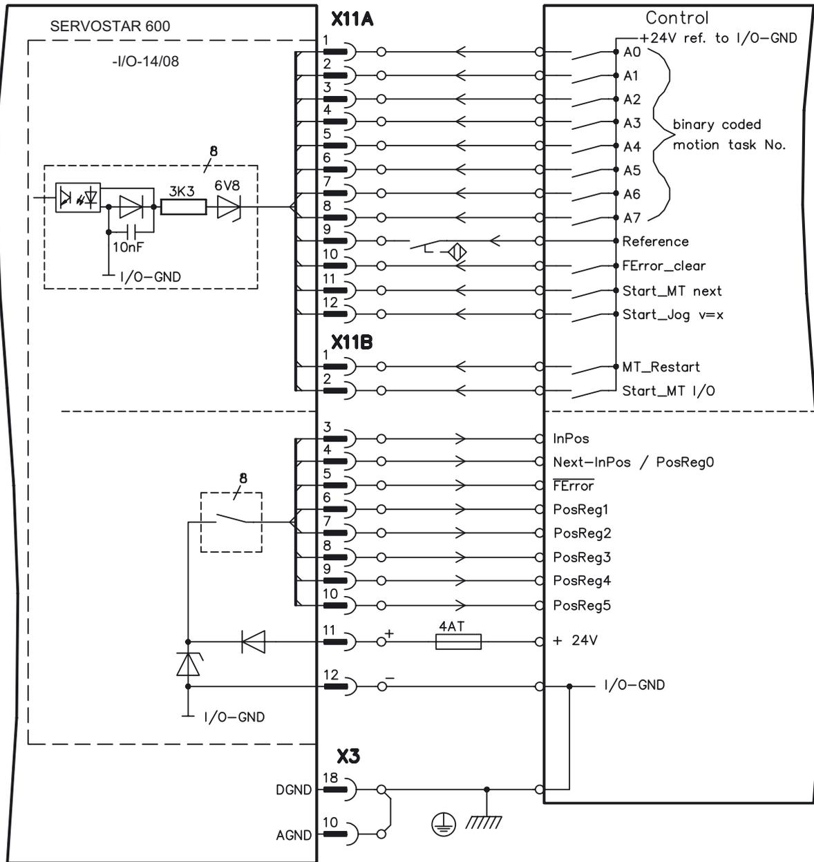
AGND and DGND (connector X3) must be joined together !
