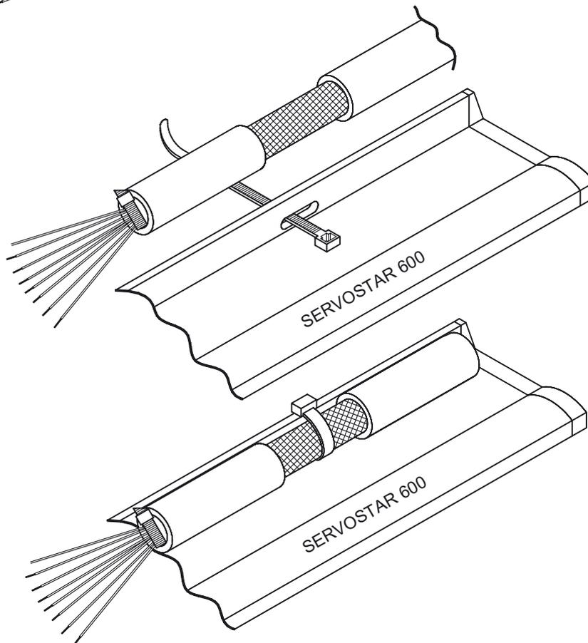
Use the cable tie to clamp the shielding braid of the cable firmly to the shielding rail.
