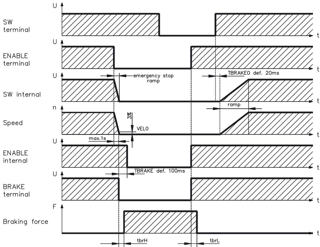
During the internal ENABLE delay time of 100ms the speed setpoint of the servo amplifier is internally driven down a 10ms ramp to 0V. The brake output is switched on when 3% of the final speed is reached. The rise (tbrH) and fall (tbrL) times of the holding brake which is built into the motors are different for the various types of motor (see motor manual). A description of the interface can be found on page 39 .
